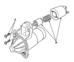
Loosen the brush holder mounting screws(A) and through bolts(B).
