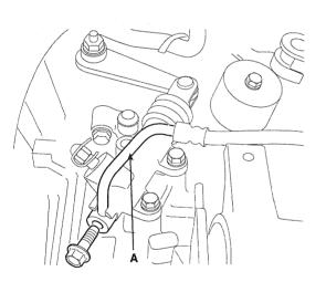
11. Install the clutch tube and clips (A).
