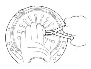
The snap ring (A) at expanded state is shown in the figure.
