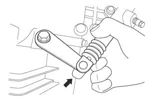
11. Install the transaxle assembly to the engine.
