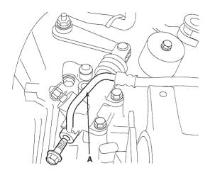
10. Temporarily tighten the flare nut by hand, then tighten it to the specified torque, being careful that the clutch hose does not become twisted.
